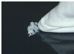
Apply AKELUX Polishing Paste to the repair area. Polish manually with AKELUX Polishing Cloth and the felt side of the AKELUX Grinding/Polishing Block or mechanically (e.g. Dremel with felt wheel).
