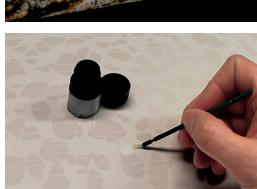
Ceramic shards that differ greatly from the decor can now be covered with a very thin layer of AKELUX Opaquing Agent. This layer must then be hardened for 60 seconds with the AKELUX LED Light Emitter\*.
