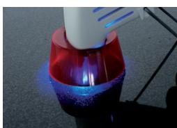
Cover with AKELUX Transparent Film/surface structure stamp\*\* and harden 60 s/cm<sup>2</sup> with AKELUX LED Light Emitter\*.
